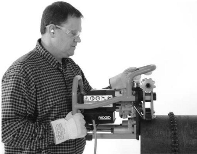
Figure 8A – Placing Beveller on Pipe
