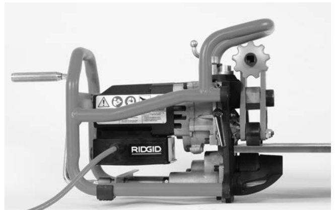
Figure 9B – Installing Beveller on Plate
