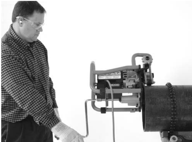
Figure 15A – Bevelling Operation
