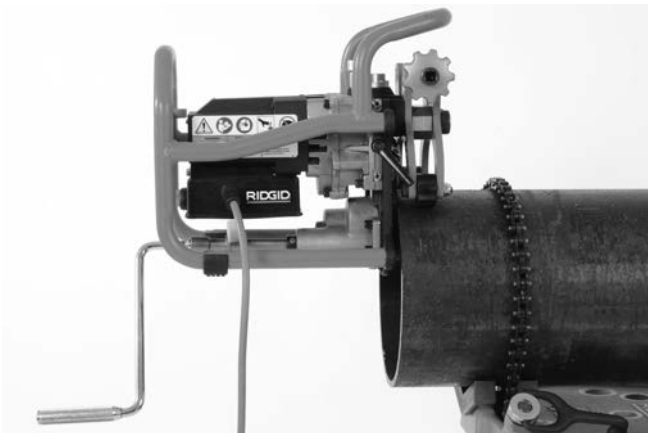
Figure 11 – Beveller Mounted On Work Piece
