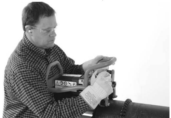
Figure 10A – Hand Tighten Clamp Screw
