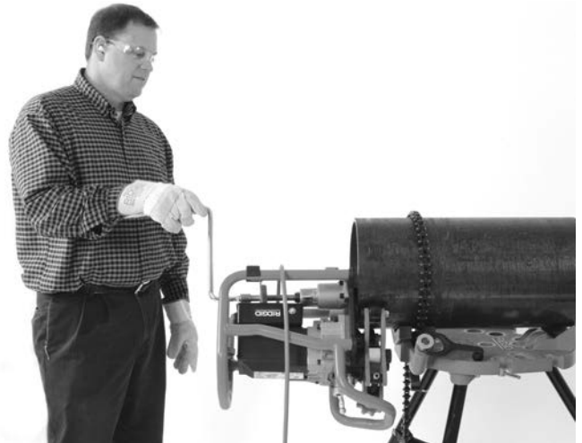
Figure 15B – Bevelling Operation
