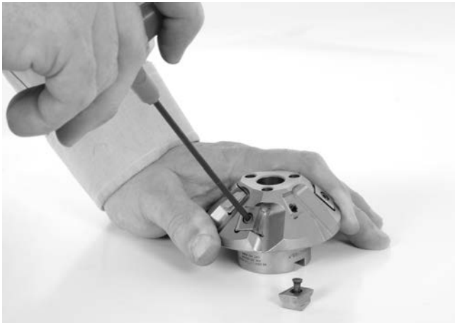
Figure 18 – Replacing Cutter Inserts
